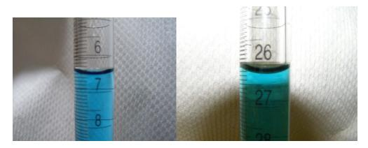
The above picture is of a burette. Note, the scale runs downward, so the reading on the left is between 6 and 7. Since the smallest increments are to the 0.1 place, the measurements should be 'guesstimated' to one more place. The above left reading should be about 6.50 or 6.55 mL. The above right reading should again be to the 0.01 place (one more than the smallest divisions) or 26.30 mL.
